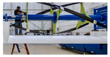
The Modular RivGen devices utilize ORPC's proven cross-flow turbine technology.
